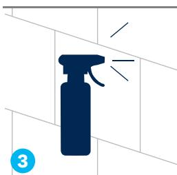
Clean the substrate with „**AKEMI Crystal Clean**“ spray (according to the manufacturer's instructions). Rinse with water and dry.
