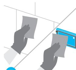
Clean the substrate and Adesio wall flange with **3M VHB Surface Cleaner** or propyl alcohol.
